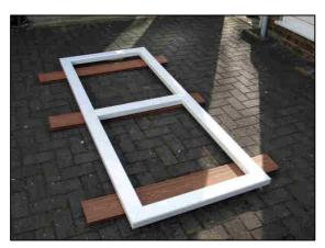
The first step will be to mark up and fit the cross braces to the welded gate frame.
