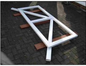
Position the cross braces underneath the welded gate frame as shown to enable them to be marked up. Each cross brace should be marked to the inside of the welded frame.
